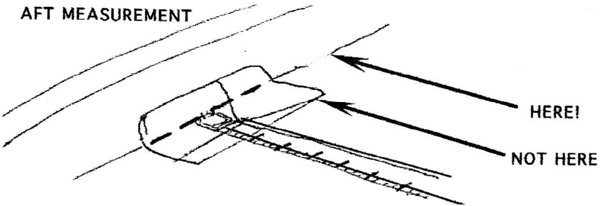
3. Measurement at the tiller hole through the transom on all classes of Bahamian boats will be measured as described in this drawing....
