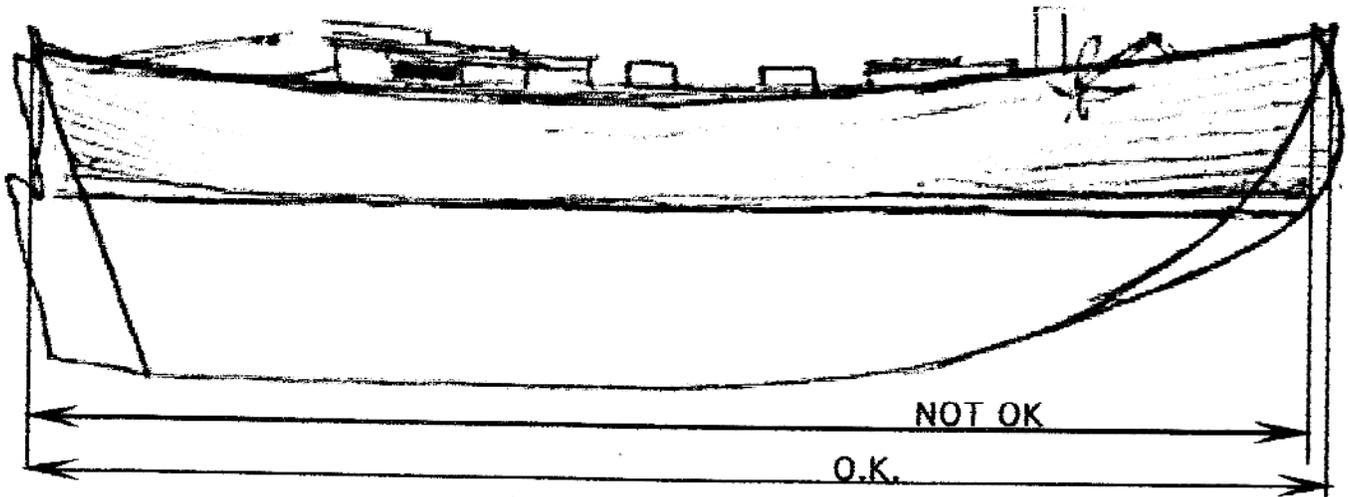
2. Any forward projection in the stem beyond plumb shall be measured and added to the overall length. Beyond this, the measurement committee may disqualify boats with extreme tumblehome, turned-back, or canoe bows even though the overall deck length complies with the above measurement.
